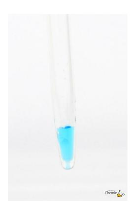
If the total nominal volume is needed, it must be made sure that a small residue is left in the pipette tip.
